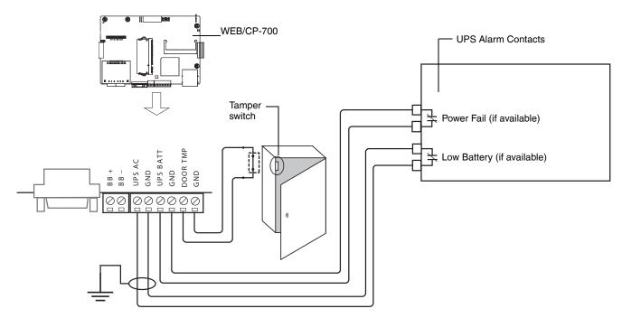
Fig. 9. Contact Input wiring to WEB/CP-700
